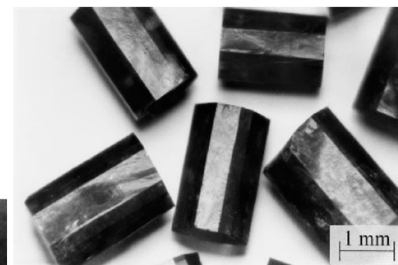
Fig. 17.9. Emerald crystals grown from \text{Li}_2\text{O}-\text{MoO}_3 flux
