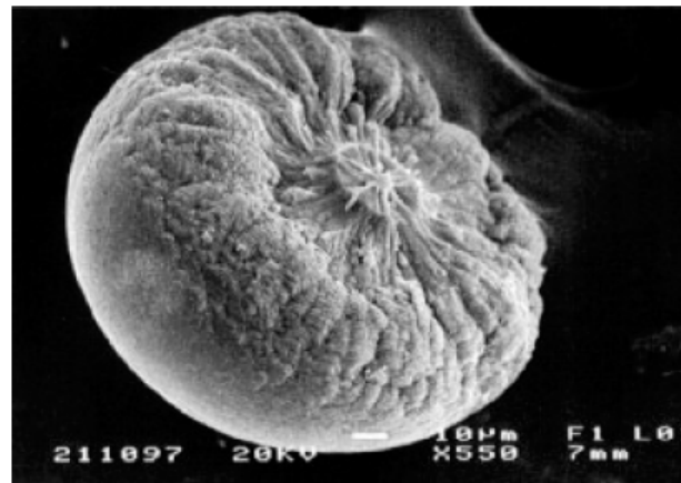
Fig. 4. SEM image showing half of an equatorially notched fluoroapatite-gelatin spheroid. Scale bar is 10\ \mu\text{m} . Reproduced with permission from Chemistry of Materials [30]. Copyright 2001 American Chemical Society.
